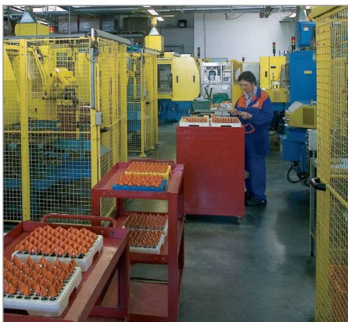
Loading the automated multi-axis CNC sharpening machines.
